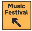
Size 1200mm x 1200mm Section 1 x-Height 127.9mm Border 28mm
