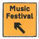
Size 1200mm x 1200mm Section 1 x-Height 127.9mm Border 28mm M11 southbound 1 mile prior to junction 12 **Q**-fit
